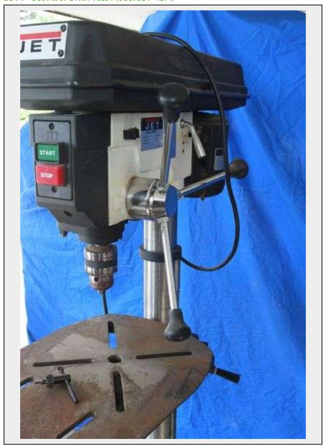
Fifteen inch swing. Spindle Speed is 200 to 3630 rpm. Motor is 3/4 HP. 115 V. Sixteen different spindle speeds. Chuck capacity is 5/8 inch. Weight is 150 pounds. Works well. Rarely used.
